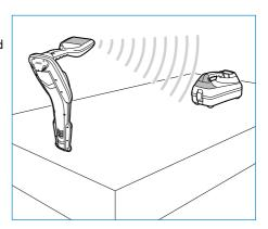
NOTE: If any iLOC commands fail, move closer to the transmitter and repeat the process.
