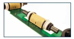
Precision by design A unique arrangement of five custom manufactured, precision ground antennas deliver locate accuracy and repeatability
