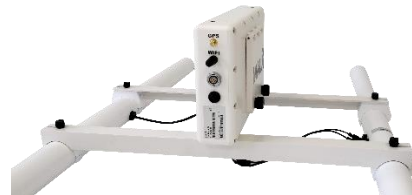
Connections for external GPS antenna and data cable together with Power On/Off on the main unit
