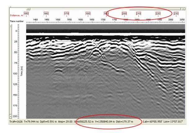
The interpretation of layers or objects is done as usual, and when saving the interpretation results the linked coordinates will join them. Most often the results are saved in ASCII format as a table readable in for instance Notepad. In the example below the depths to two layers are shown, Layer 1 and Bottom.
