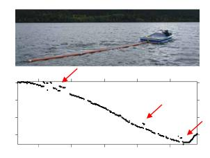
measured line. It might sometimes be better to only measure the breakpoints and then interpolate the positions in-between, as shown above. This is applicable if measurements are performed in straight line segments between the breakpoints.
