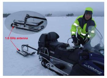
In the picture above the antenna is attached to a simple wagon, and then to the towing hook of the car. To the left an example is seen how the antenna can be attached to a snowmobile and where the CX main unit is kept in the front of the snowmobile. The GPS antennas are in these cases located in a plastic box on the snowmobile and on the roof of the car.
