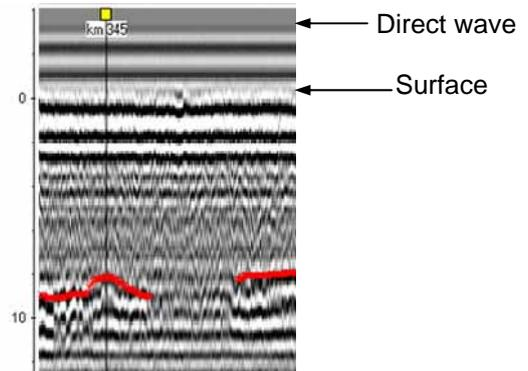
The data also clearly shows the structure of the ballast material, as an uncountable number of small hyperbolas.
