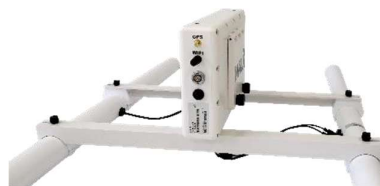
Connections for external GPS antenna and data cable together with Power On/Off on the main unit
