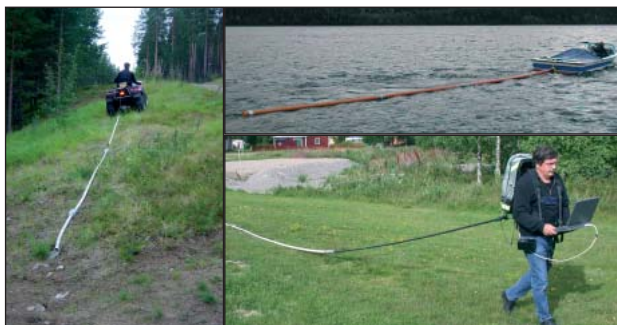
Figure 3 Different applications of the RT antenna. When measuring on water the RT antenna is placed within a plastic tube.
