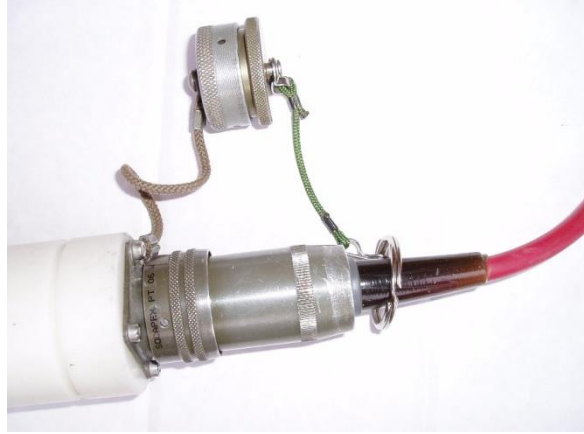
Figure 47 Connecting the dust caps
