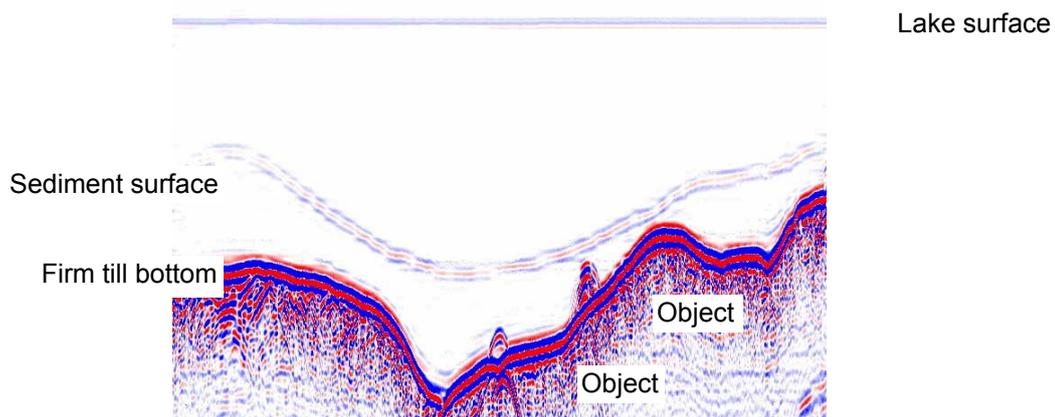
The following pictures, created with Surfer, represent the track measured together with two maps of the different identified depths. In the middle the depth to the firm bottom is shown (in m) and to the right the depth from lake surface to sediment surface. The colour scale represents a depth range from 2 m (gray) to 11 m (black). These two can then be used to calculate the thickness and amount of the sediment.
