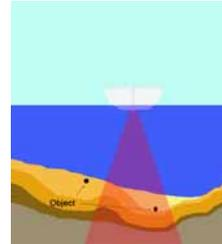
It should also be noticed that the antenna footprint in water is smaller than in other geological medias.
