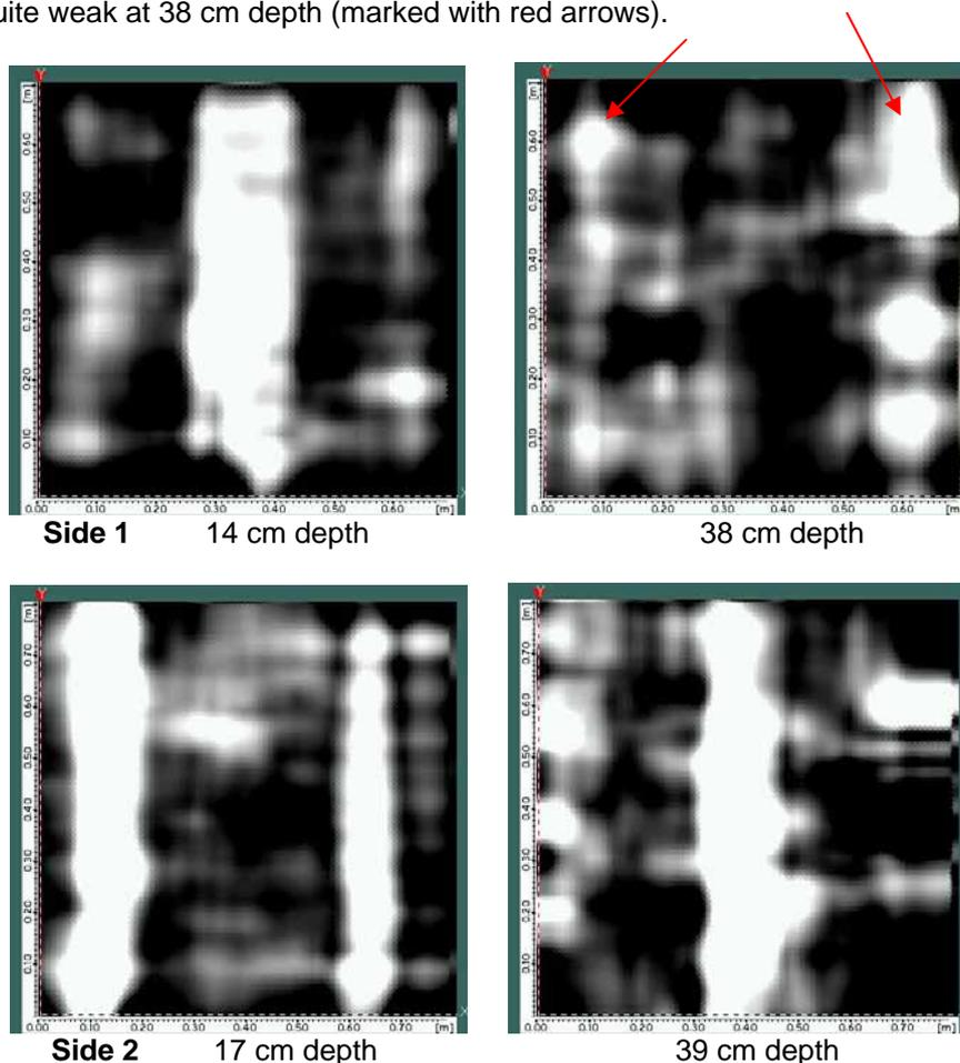
At side 2 the reflections of the pipe closest to side 1 is as strong as measured from side 1 indicating a difference in material. This pipe, as seen above, contains the aluminium pipe with a diameter of approximately 5 cm.
