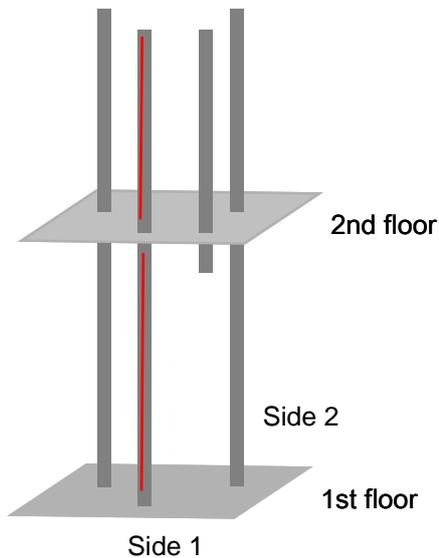
A simple drawing of the pipe location at 1<sup>st</sup> and 2<sup>nd</sup> floor is given at left. As seen the pipes on side 2 goes through both floors, while one of the pipe on side 1 only goes through the second floor. The chimney contains 6 pipes in total, so the two missing pipes in the picture at left are only going from top of the 2<sup>nd</sup> floor and up.
