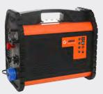
With up to 60 A output current it enables even deeper soundings with larger transmitter loops.
