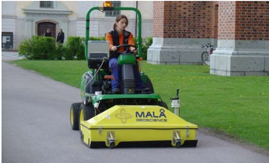
Figure 5. A suitable mounting of the array system on a lawn-mower type of vehicle.
