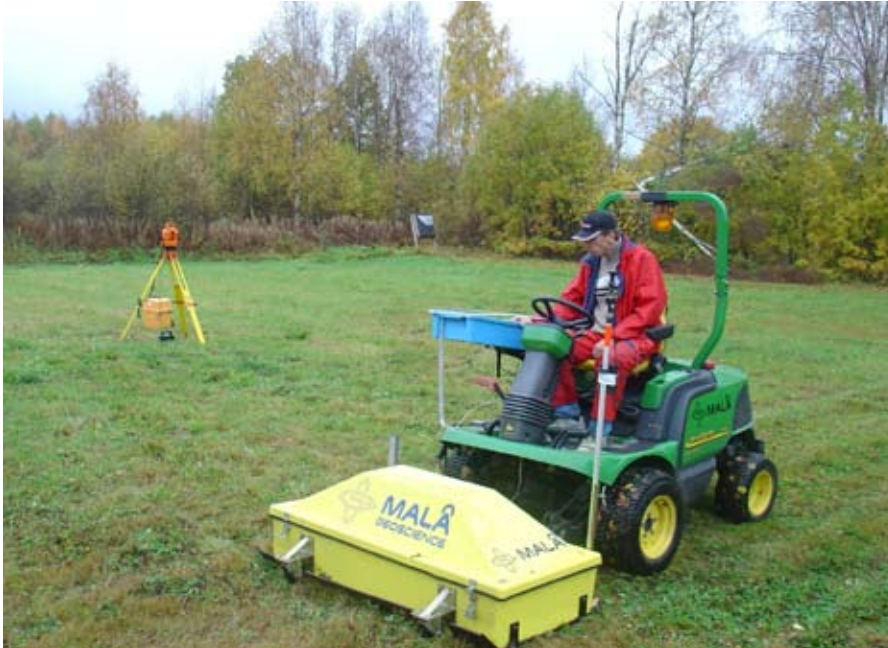
Figure 7. Data acquisition with a 400MHz array, the total station is seen in the background
