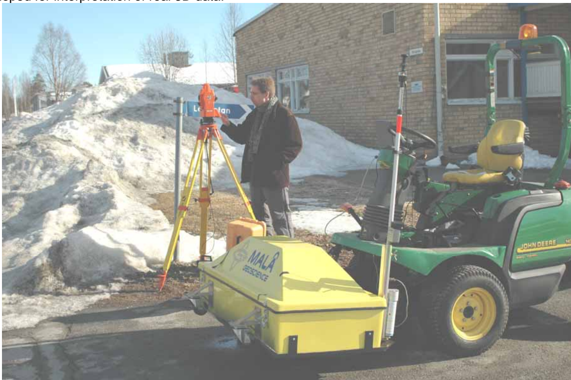
Figure 1. Equipment used: radar array (mounted on a John Deere tractor) and a total station.
