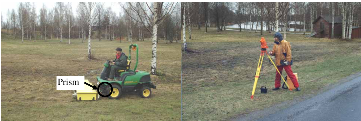
Figure 2. During the survey the total station tracks the prism located on the antenna array.
